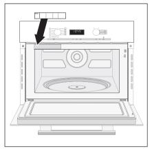
Stick the enclosed short instructions to the frame behind the door as illustrated, making sure they do not block any of the vents. The appliance must be built in before it can be used. Otherwise it poses an electric shock hazard.
